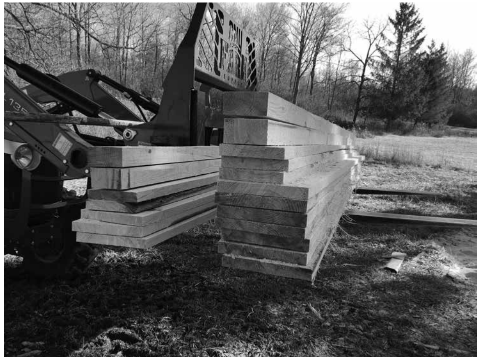
Figure 2. Lumber produced from two 10 foot logs of identical age. The lumber on the left, 44 board feet, was produced from a log that was 10" on the narrow end. The lumber on the right, 75 board feet, was produced from a log that was 12" on the narrow end.
