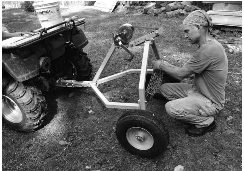
Author with ATV and miniature log arch. Despite its small size and bargain price, this arch has proven to be both durable and effective in its operation. Photo courtesy of Jeff Joseph.
