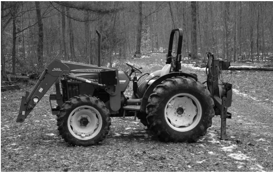
Figure 4. Tractors were not designed to work in the woods (skidders are designed for woods work). The relatively high center of gravity of tractors necessitates extra effort to avoid problems (via planning and awareness) and protections if a problem develops. The Roll Over Protection System (ROPS) when the seat belt is used helps reduce the likelihood the operator is crushed if the tractor rolls over.
