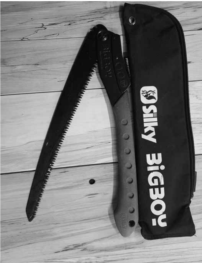
Figure 4. Folding saws find numerous tasks. Smaller saws can easily slip into a hip or side pocket. Larger saws, such as the 15" saw pictured, can fit in most day-packs and handle larger stems.
