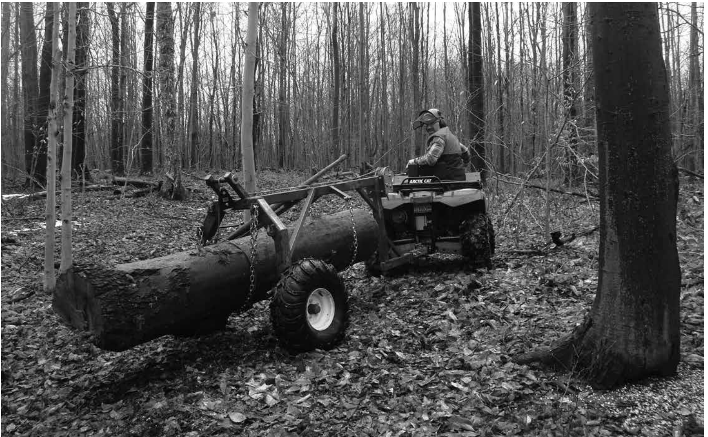
Figure 6. Logging arches are used in small-scale low impact situations to move single logs. Production is low, but for the occasional easy-to-access log, this works well. The log is kept clean for the sawmill or cutting into firewood.
