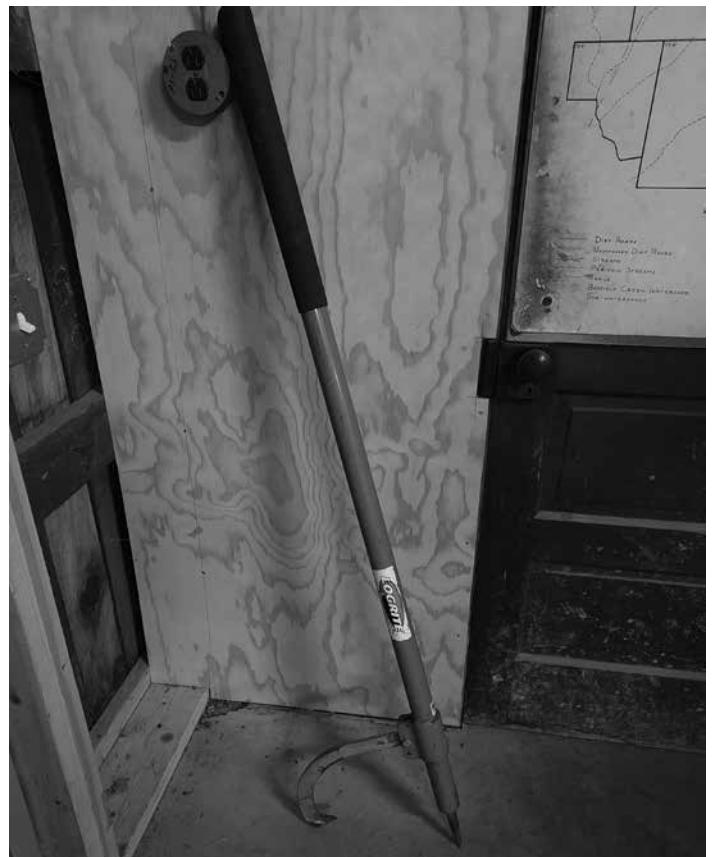
Figure 3. The peavy had its start in the logging industry. The basic design is unchanged, although a variety of materials are used. This tool excels as a lever to maneuver logs into position or for releasing a pinched chainsaw bar.
