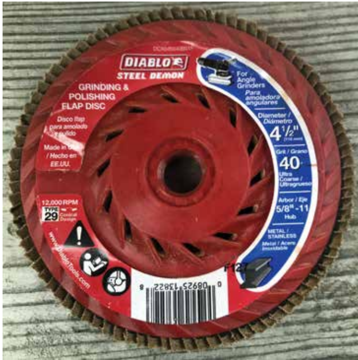
Figures 3, 4. Using a flap disc on an angle grinder is an effective way to remove bark while doing minimal damage to the wood beneath.
