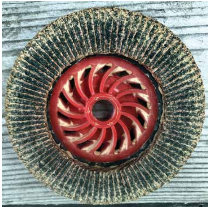
Figures 3, 4. Using a flap disc on an angle grinder is an effective way to remove bark while doing minimal damage to the wood beneath.
