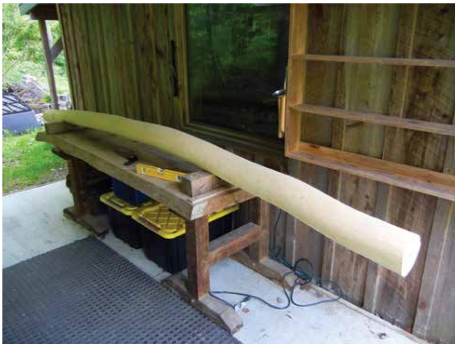
Figure 5. Stout sawhorses and a pair of 4x4s with v-shaped notches cut into them helped stabilize the pole while removing the bark and cutting it to length.
