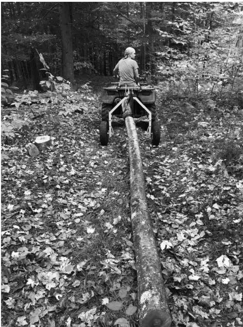
Figure 2. Dragging out the black birch pole with ATV and small log arch.
