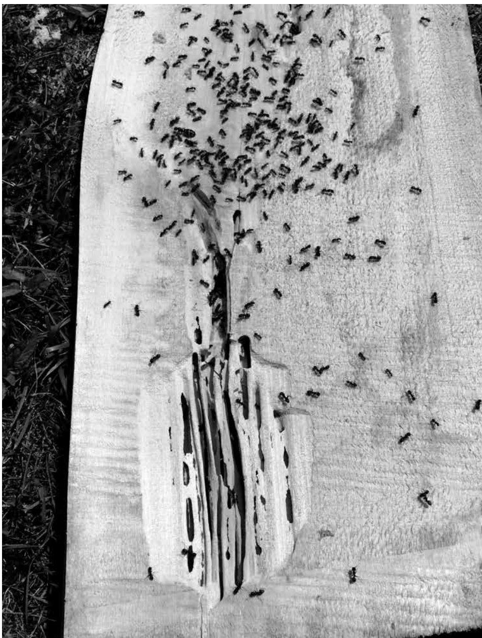
Figure 2. Disturbed carpenter ant colony in basswood board.
