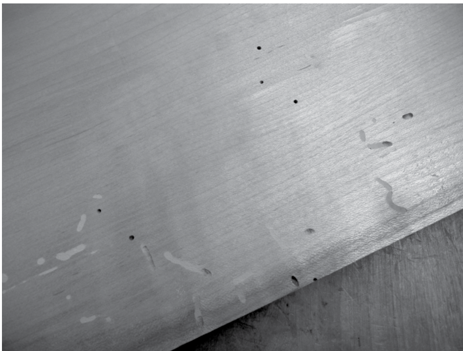
Figure 3. Powder post beetle damage in maple board.
