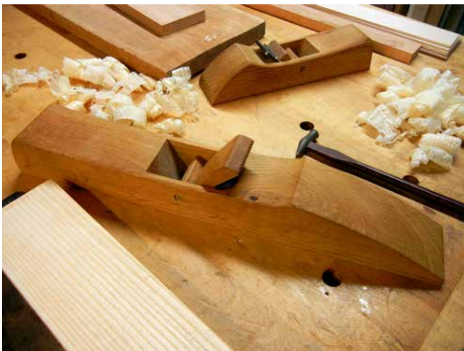
Figure 5. The wood-bodied jointer plane in the foreground was made of a discarded white oak remnant from a timber framing project; in order to ensure its stability, the block used to create it was first rough-milled and left to air dry for over three years before being put to use.
