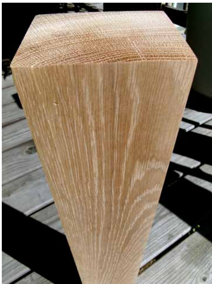
Figure 2. White oak, flatsawn face. Note the strong contrast between the early and latewood on both end and face grain. The medullary rays on this face are seen only as faint and narrow parallel lines. The wide pores in the early grain give oak lumber a characteristically coarse surface, even after sanding or planing.
