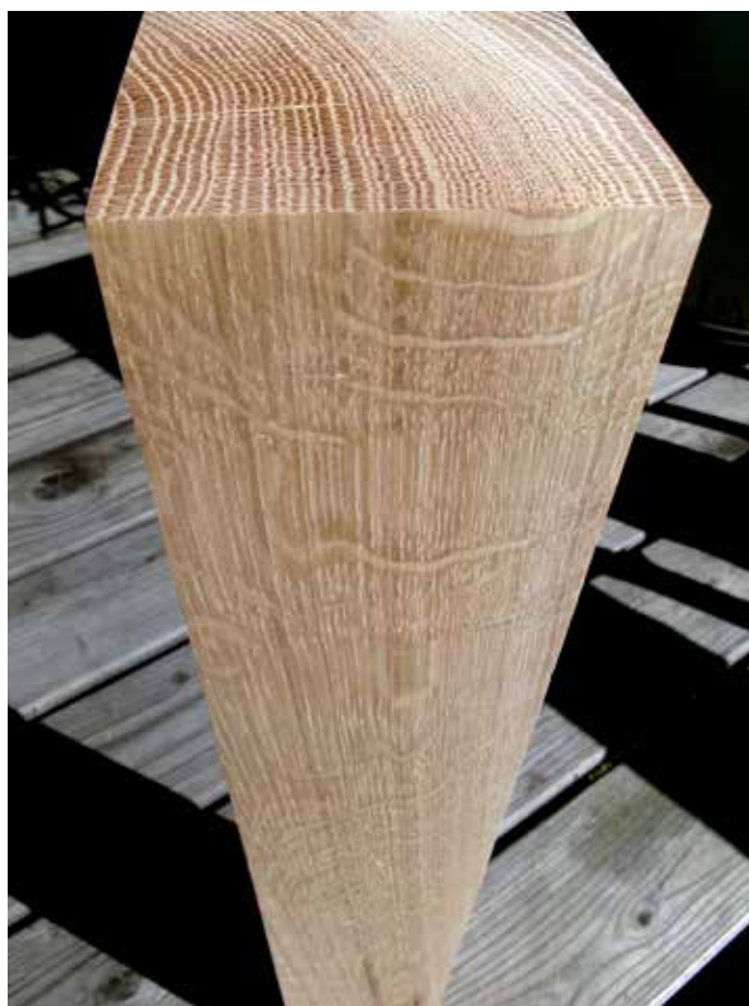
Figure 3. White oak, quartersawn face. Note the very prominent medullary rays running perpendicular to the grain direction of the wood. Quartersawing white oak, by cutting on the radial plane, creates lumber with ‘vertical’ grain, accentuating the rays in cross-sectioned bands in oak. The Arts and Crafts and Mission styles of furnituremaking have used this figure to great effect.
