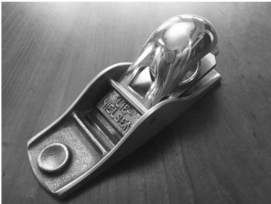
Lie-Nielsen No.102 low-angle block plane; an American-made and heirloom quality tool.
