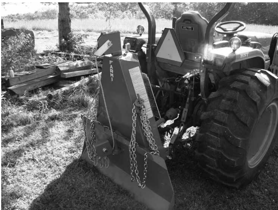
Figure 3. PTO driven winches attached to a farm tractor allow logs to be pulled to the tractor. The tractor then drags them to where they can be processed. Except on snow or ice, the logs usually accumulate dirt and debris in the bark which will dull your chainsaw.
