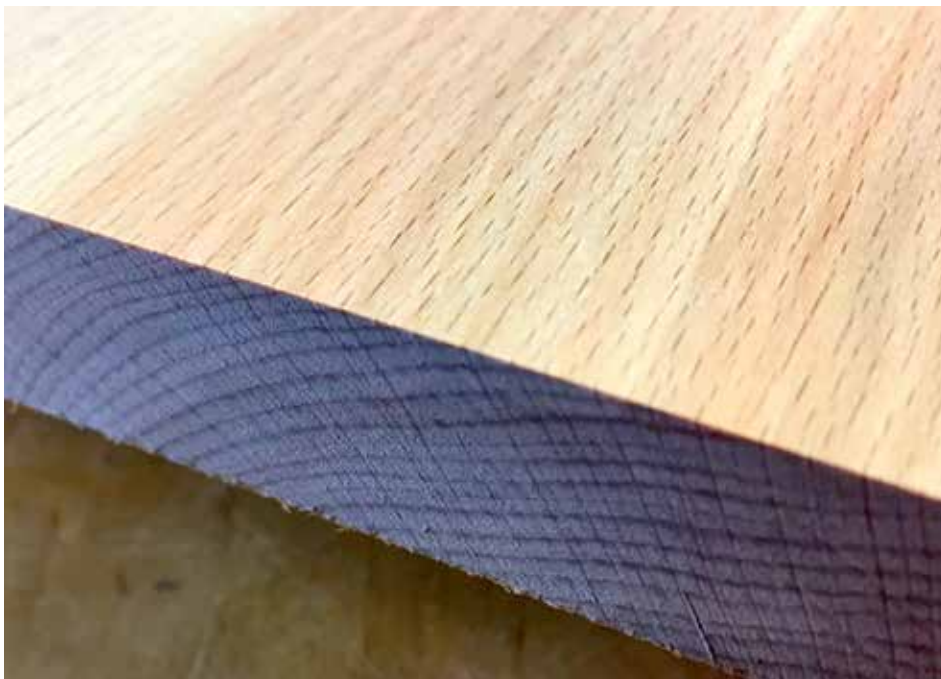
Figure 6. The endgrain of this rift-sawn beech board shows +/-45 degree growth rings, with the clearly visible rays running in a perpendicular direction to the annual rings.
