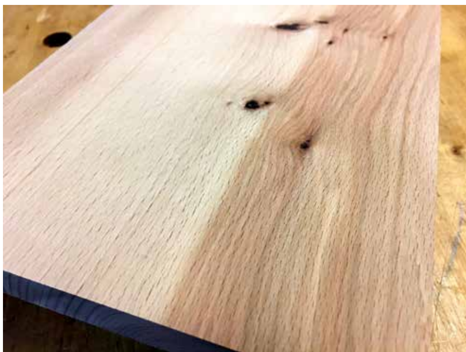
Figure 4. Beech board with contrasting bands of light sapwood and darker heartwood; small diameter knots are a common defect.
