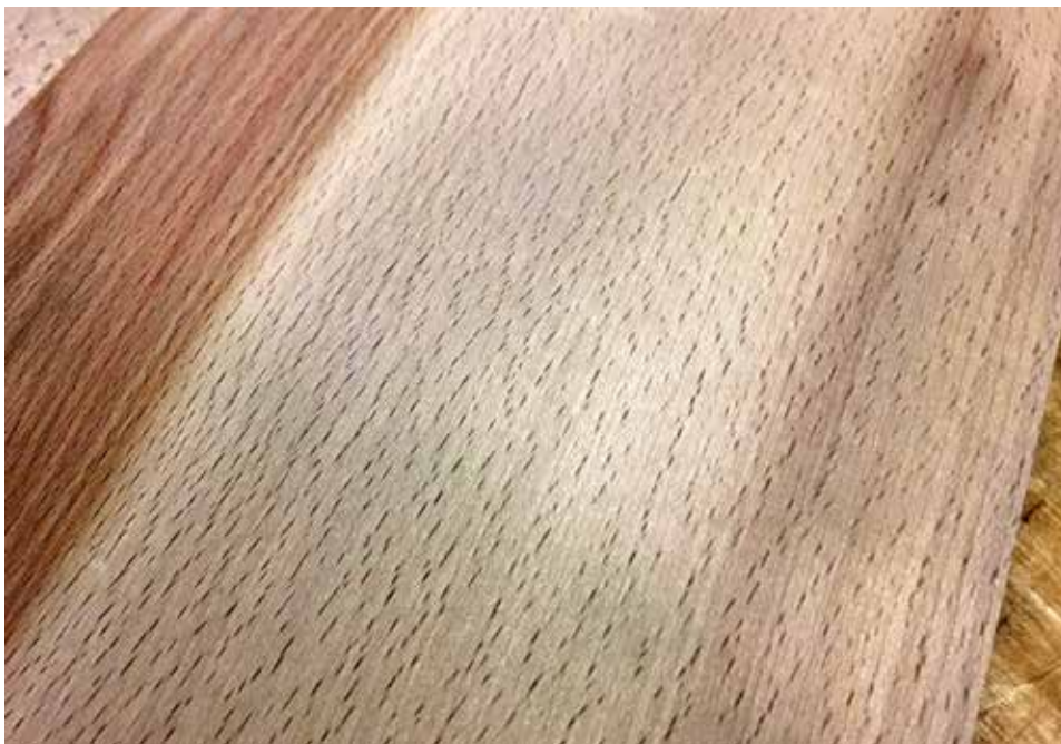
Figure 8. Unlike most hardwoods, in beech the medullary rays are also highly visible on the flatsawn faces of boards, seen here as dark dashes against the contrasting wood grain.
