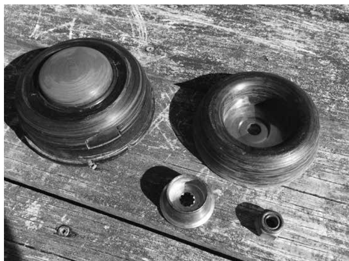
Figure 2: To install a trimmer blade, first remove the bump feed head (left) and use the appropriate adapter kit designed for the purpose (right).
