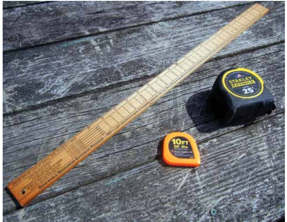
Big tree hunting toolkit: a Biltmore stick, diameter tape, and standard tape measure. Serious hunters may want to invest in a laser distance meter to accurately measure tree height.
