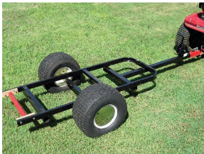
The trailer frame with tires and tow bar.
