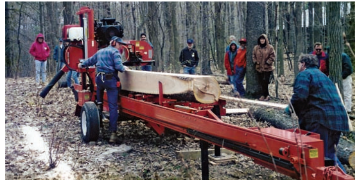
Ron & Judy De Witt demonstrate portable band mill operation during a woodswalk on Patty Kay & Ken Rayna's property in Galway, NY, in 1998.
