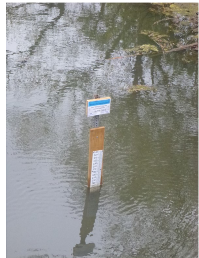
This water level gauge indicates the amount of surge from Lake Erie.
