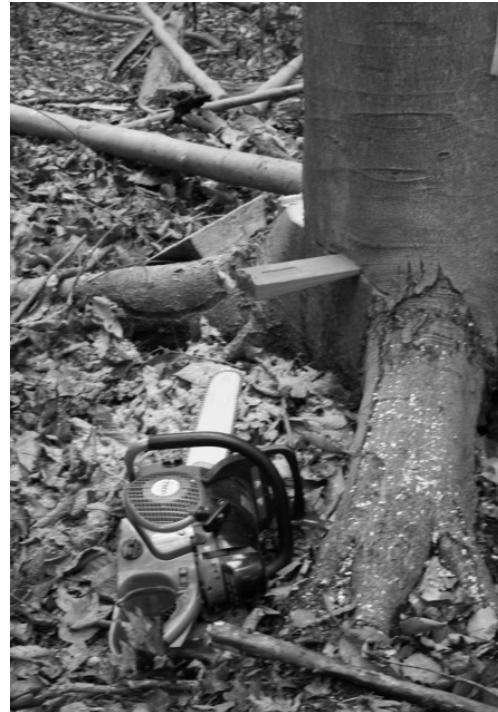
A chainsaw and felling wedge are useful tools for cutting trees
