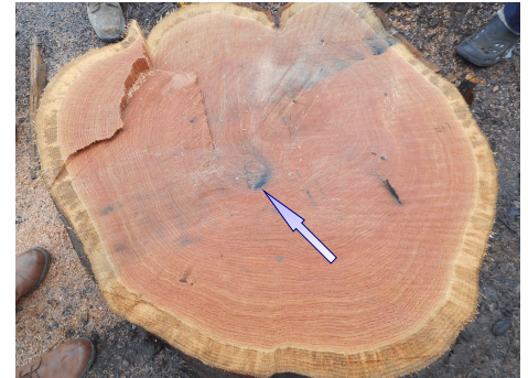
Metal detection in timbered logs is noted by the dark stain deep within the tree.
