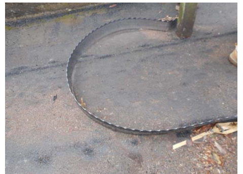
Undetected metal destroys saw blades.
