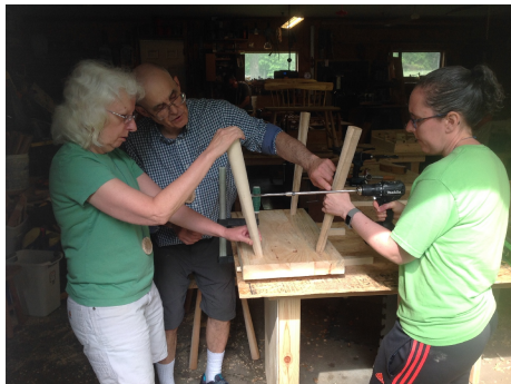
Dave Abeel explains to Sara and Jan the importance of lining up stretcher tenon holes for front and back legs on Sara's boot bench.
