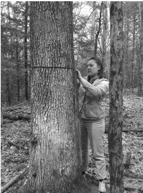
Figure 3. A diameter tape is wrapped around the circumference of the tree, and the unique calibration allows direct recording of tree diameter. A 3.5 ft staff is placed on an aluminum nail about 1 ft above the ground for accurate repeated measurement.
