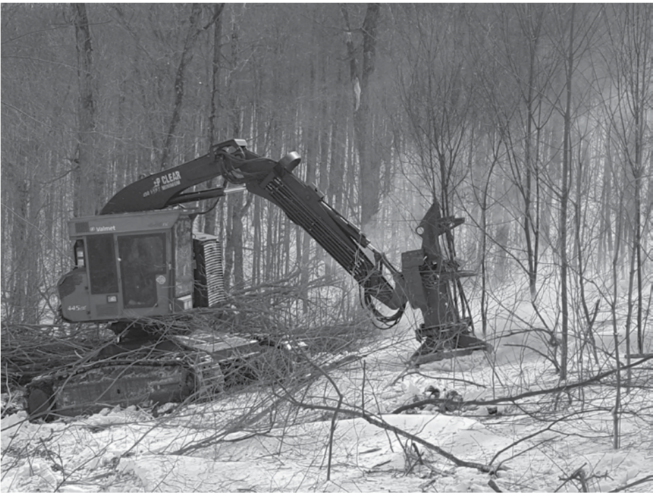
Figure 4. A feller-buncher can efficiently clear the understory, although it is most commonly used in harvesting larger trees. The cutting head allows for stems to be bunched at specific locations.
