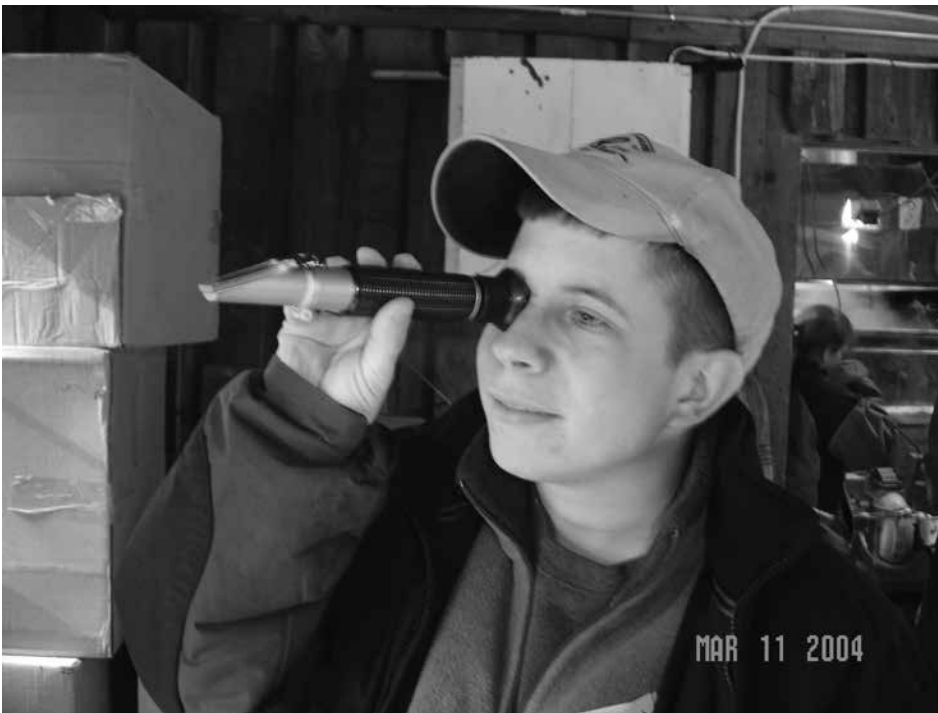
Figure 6. Refractometers are an accurate way to test the concentration of solids (sugars) in the sap to determine when it becomes syrup.
