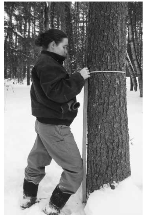
Figure 4. Repeated accurate diameter measurement of this white pine is simplified by an aluminum nail at approximately 12 inches above ground and a 3.5 ft stick.
