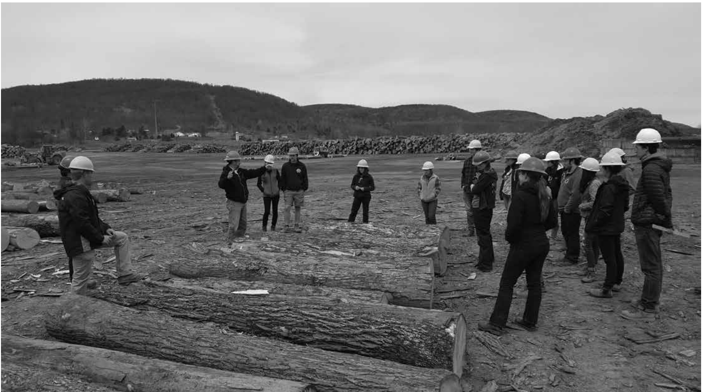
Figure 1. Tom Gerow of Wagner Hardwoods explains log scaling and grading to students. Purchased logs are arranged in the log yard to facilitate viewing the log for features of quality and defect (i.e., grading) and to measure log length and diameter of the small end.
