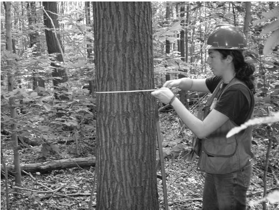
Figure 2. Estimating the volume of a tree begins with measuring diameter. The most accurate measurement is obtained with a diameter tape, or “d-tape” as pictured. Scale sticks and ocular estimation also provide estimates of tree diameter.
