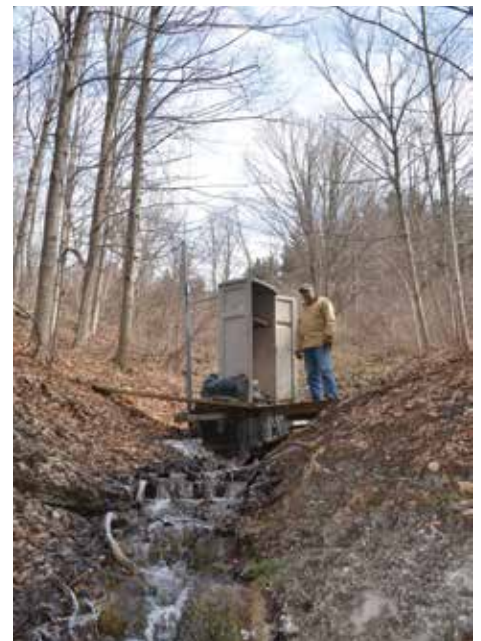
Peter inspects a microhydro gauging station used to support their net-zero renewable energy system. Multiple streams on the property with drop in elevation allow for harnessing the power of water.
