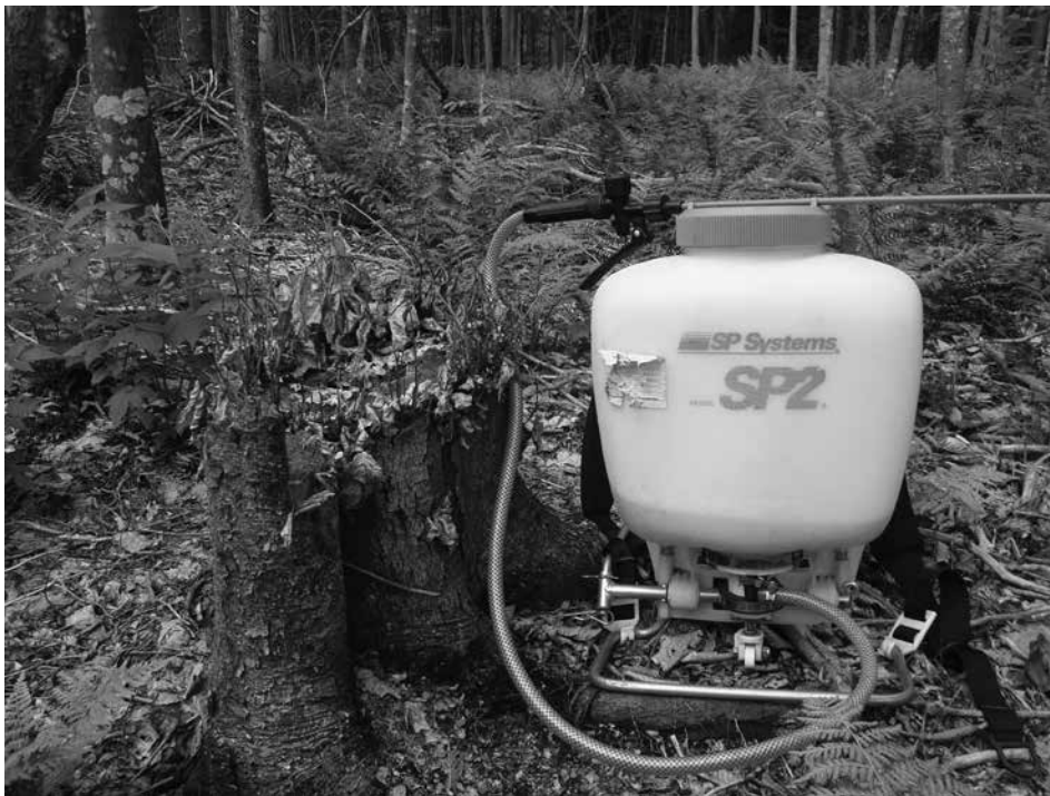
Figure 4. Backpack sprayers are inexpensive and handy tools for applying foliar, basal bark, and cut-stump applications of herbicide. Knowing the correct mixing concentration will reduce waste and minimize unnecessary applications of herbicides. This sprayer holds approximately 3 gallons, the V 2 used in Formula 2.
