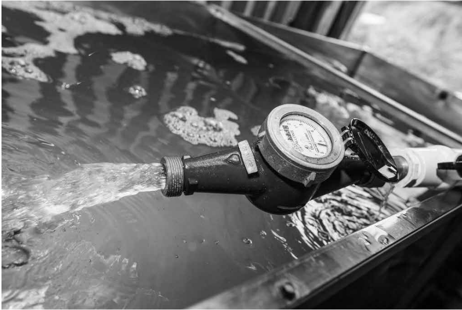
Figure 3. The sap seller and buyer will need to be able to accurately measure sap sugar concentration and sap volume. A totaling meter is the most accurate method to determine the
