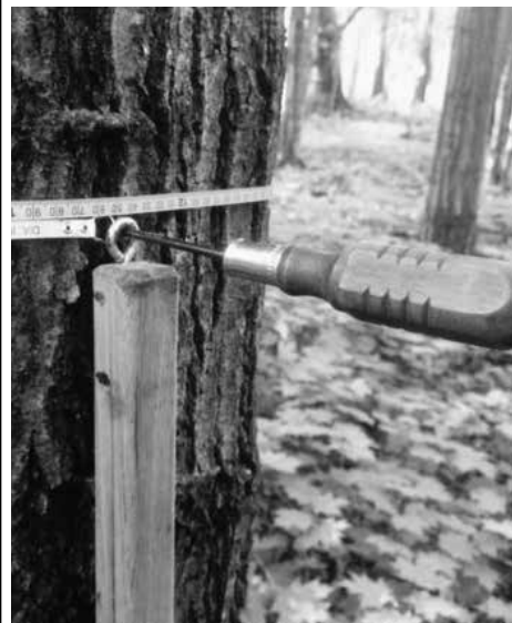
After placing the awl through the eye hook and DBH tapes loop, you can walk around the tree to accurately measure the DBH.
