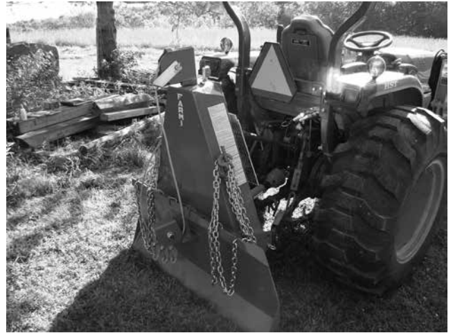
Special attachments for ATV and tractors, shown here with a winch, increase safety and productivity. Care is needed if these types of machines are used for small scale logging.
