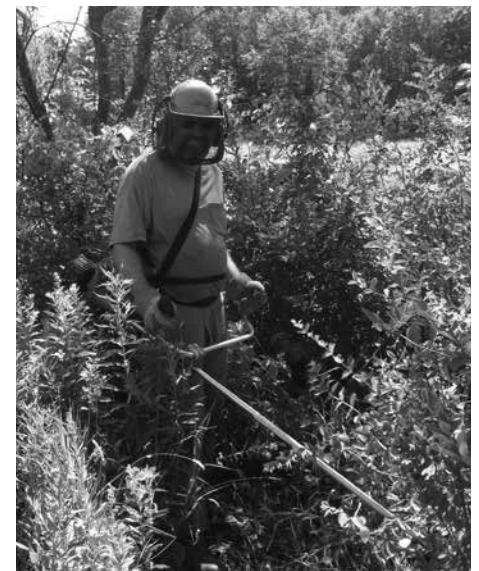
Brush saws can be used as a selective mechanical treatment, or combined with a herbicide to the freshly cut stump to limit sprouting. Personal protective safety equipment is essential.
