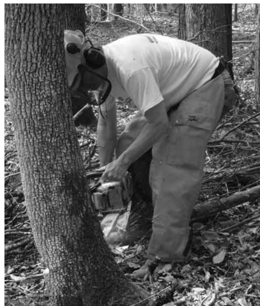
Notice the chaps on the individual using the chainsaw.
