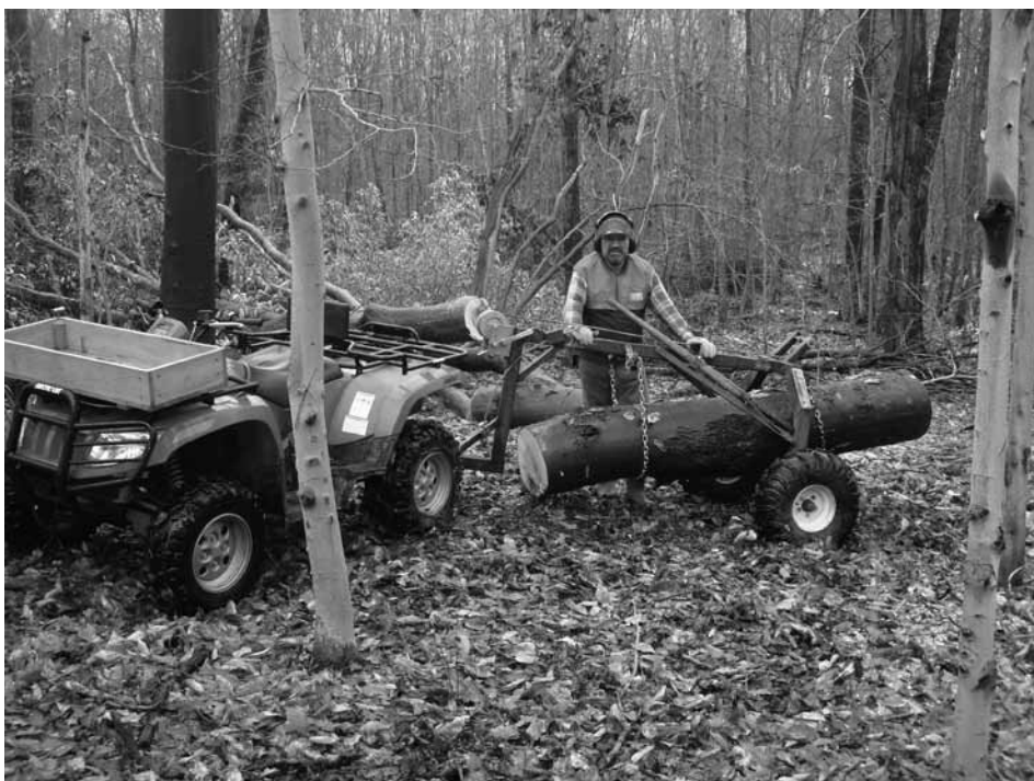
An ATV and arch can move firewood logs either suspended (as shown) or skidded. Careful planning and operation will control damage to residual trees, avoid rutting, and minimize effort in the woods.
