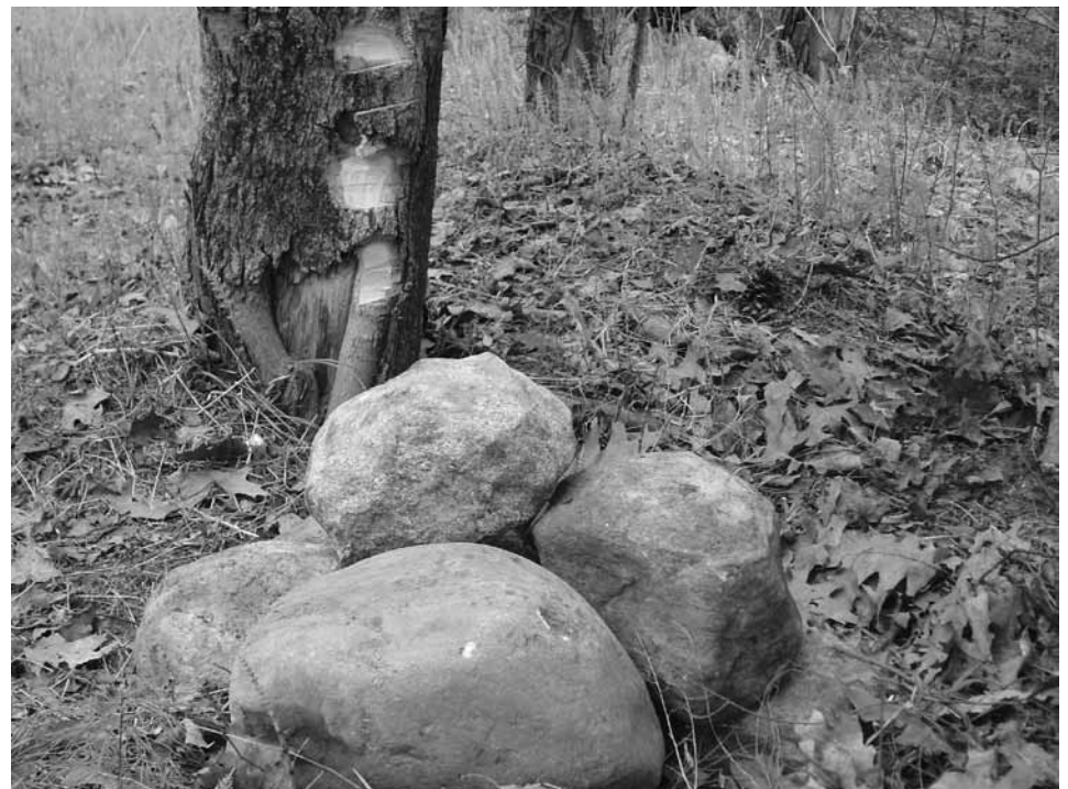
A corner monument, in this case rocks that bury a 4 foot iron pipe, is marked using three blazes in vertical sequence and painted with a bright fluorescent color.
