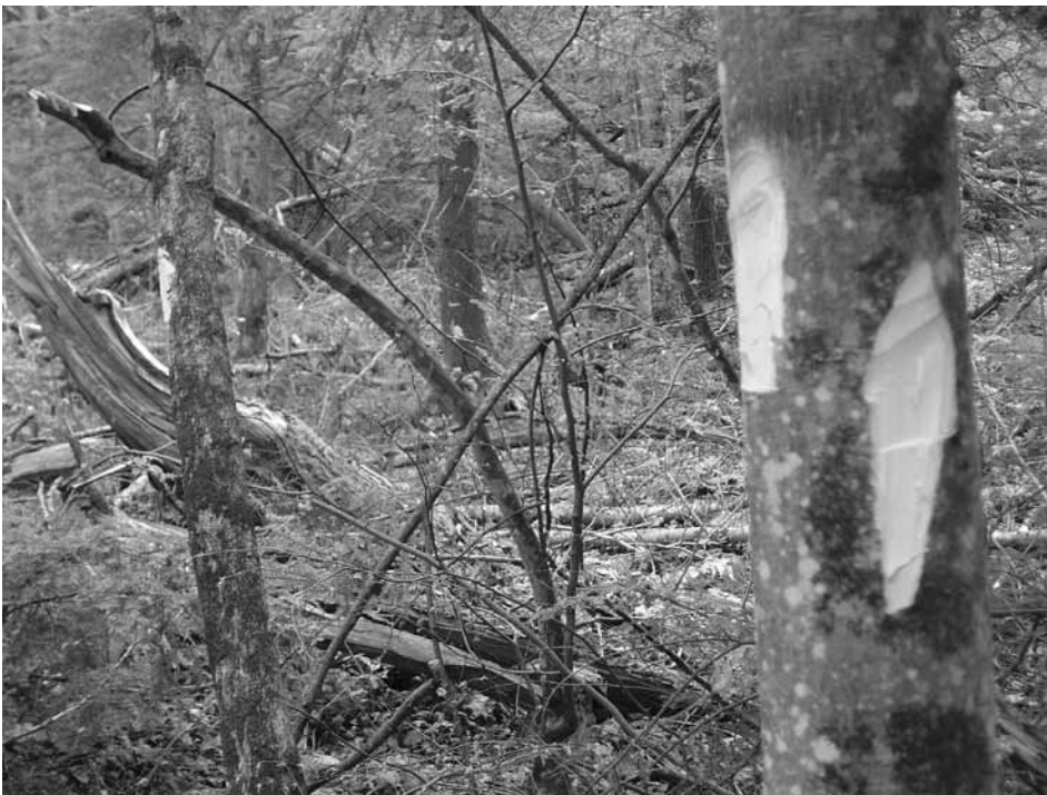
Blazes on a tree indicate the proximity of the tree to the boundary line. In this case, the tree is blazed and painted to indicate it is within one foot of the boundary line.
