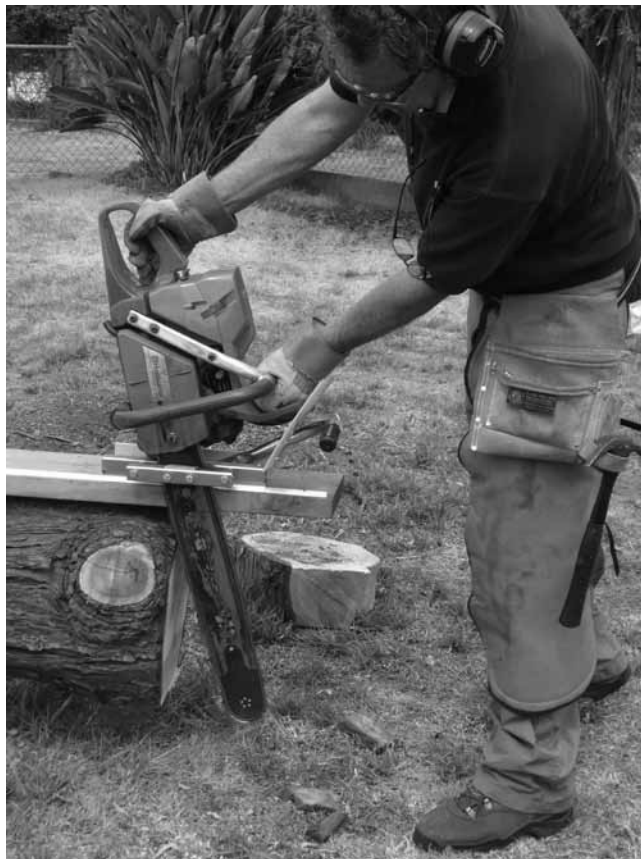
Chainsaw mill frame attached to a suitable chainsaw showing v-groove on a straight edge.
