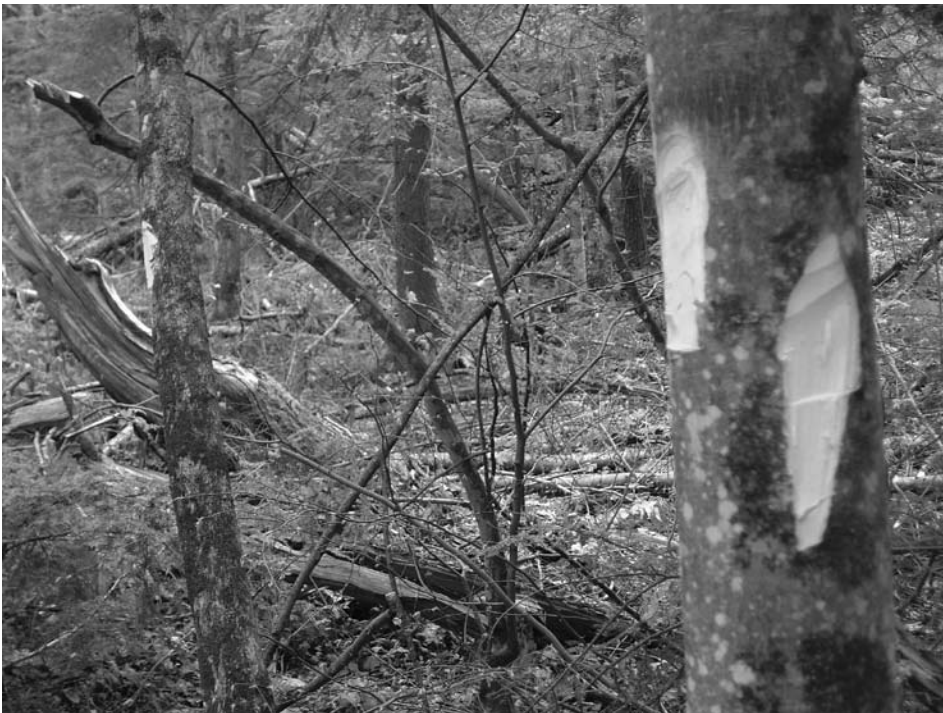
Blazes on boundary line trees should be at approximately eye level. The blaze is made with a small hand ax or hatchet and removes the bark for hand-sized or slightly larger patch. Don't blaze high value trees. Use correct survey protocols for selection of trees and placement of the blaze. Avoid spring time for blazing and painting so weeping sap doesn't flush away the paint.
