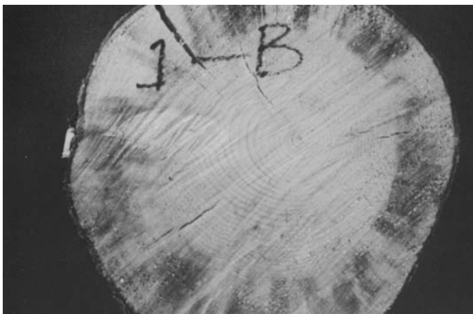
Figure 1. Cross section of a pine log showing sapwood darkened by a blue stain.
