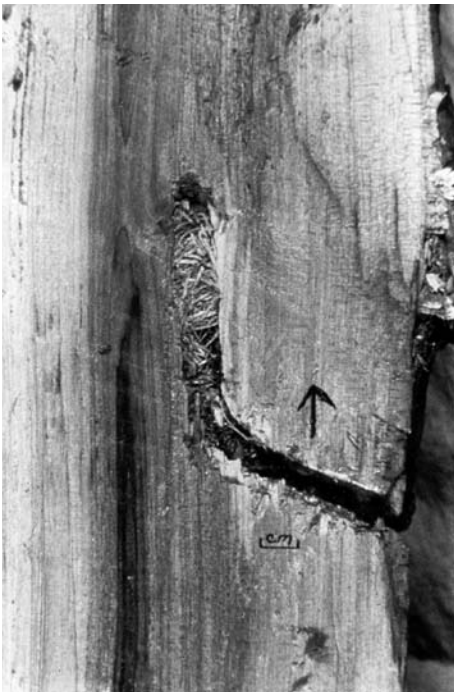
Figure 3. An over-wintering gallery of maple borer and associated mineral stain. The latter is indicated by the dark-colored wood surrounding the gallery. The arrow indicates the orientation of the log.
