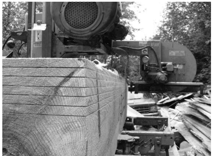
Thin kerf bandsaws remove only about 1/8th inch with each cut — increasing yields significantly.
