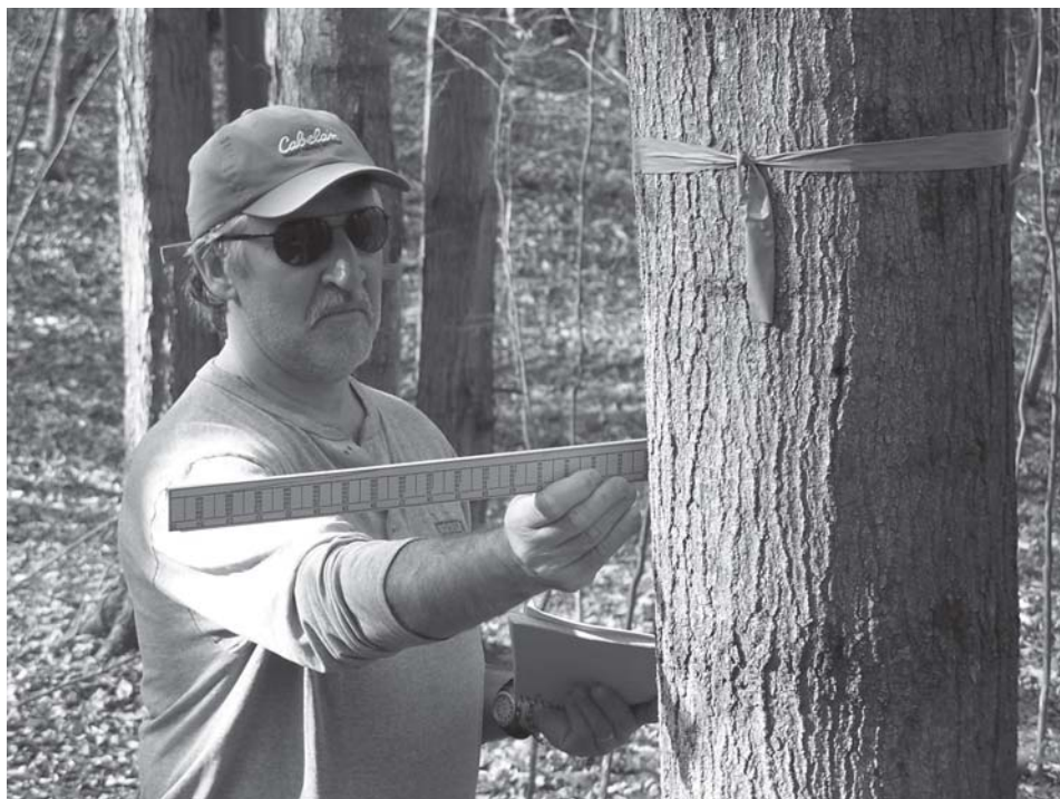
A scale stick can be used to measure both tree diameter and merchantable height of a tree. The scale stick also has a volume table that helps estimate the number of board feet.
