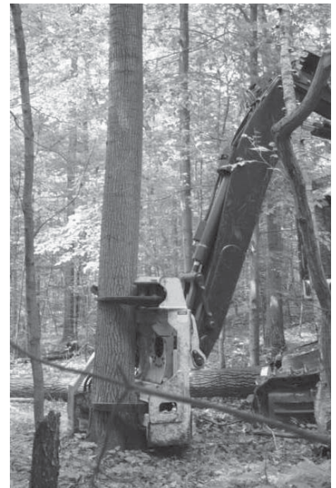
Cutting a tree with the feller/buncher.
