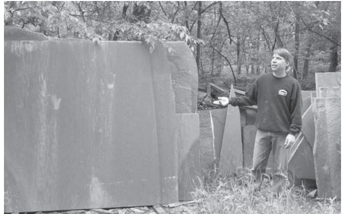
Bill Mirch with large block of bluestone for sawing into dimensional pieces.
