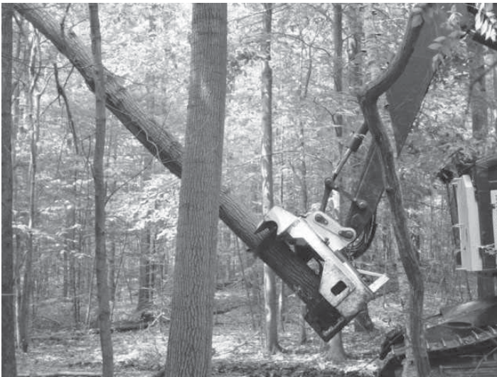
Felling a tree with the feller/buncher.
