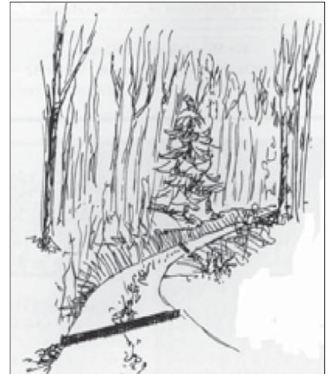
Flexible Belt Culvert
