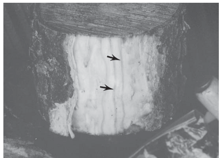
Figure 2. This is a section of black cherry showing defects caused by Phytobia on the surface of the sapwood (arrows).
