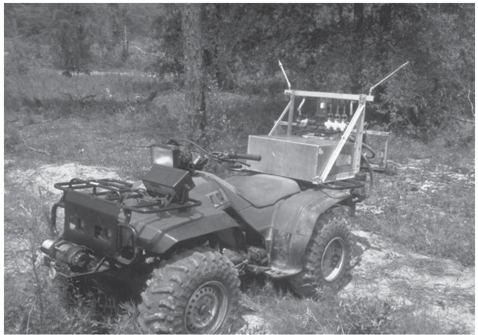
ATVs and similar machines can be outfitted with equipment, like herbicide applicators or cutting heads, to aid in treating vegetation. Photo: David J. Moorhead, The University of Georgia, www.forestryimages.org
