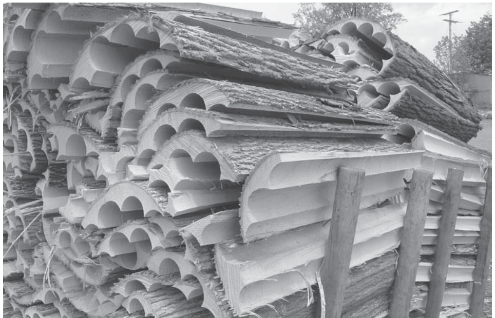
A stack of ash wood that remains following removal of cores for baseball bats.
