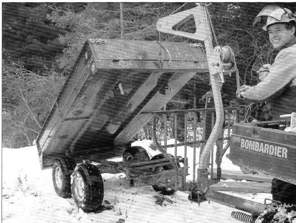
Bombardier ATV towing a Nova Jack trailer with the dump box attachment. Bill Lindloff, of Pro-Cuts and a Game of Logging instructor is demonstrating how to operate it. Photo: Brendan Kelly,
