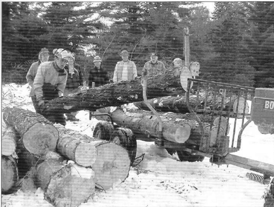
Bombardier ATV towing a Nova Jack trailer with a load of white pine. Bill Lindloff is demonstrating how to operate the loading/off loading pivot system. Photo: Brendan Kelly
