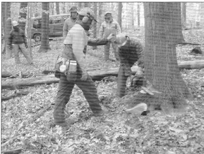
Bill Linloff is about to advise participant (John Miller) that the face cut needs to be more open, greater than 70 degrees.
