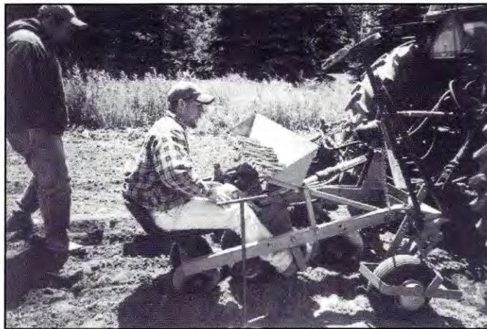
The Frobbesta plants 10-inch cuttings at the rate of one-half acre per hour.
