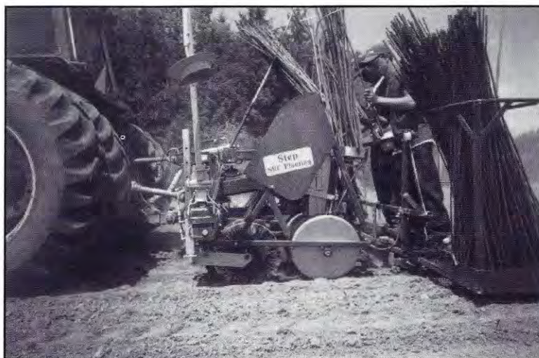
The new Step Planter plants two double rows at a rate of 2 acres per hour.
