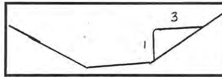
Inset: Cross Section of Level Portion. This slows the water and forces runoff to spread out in the channel. Rock- or sod-lined.
