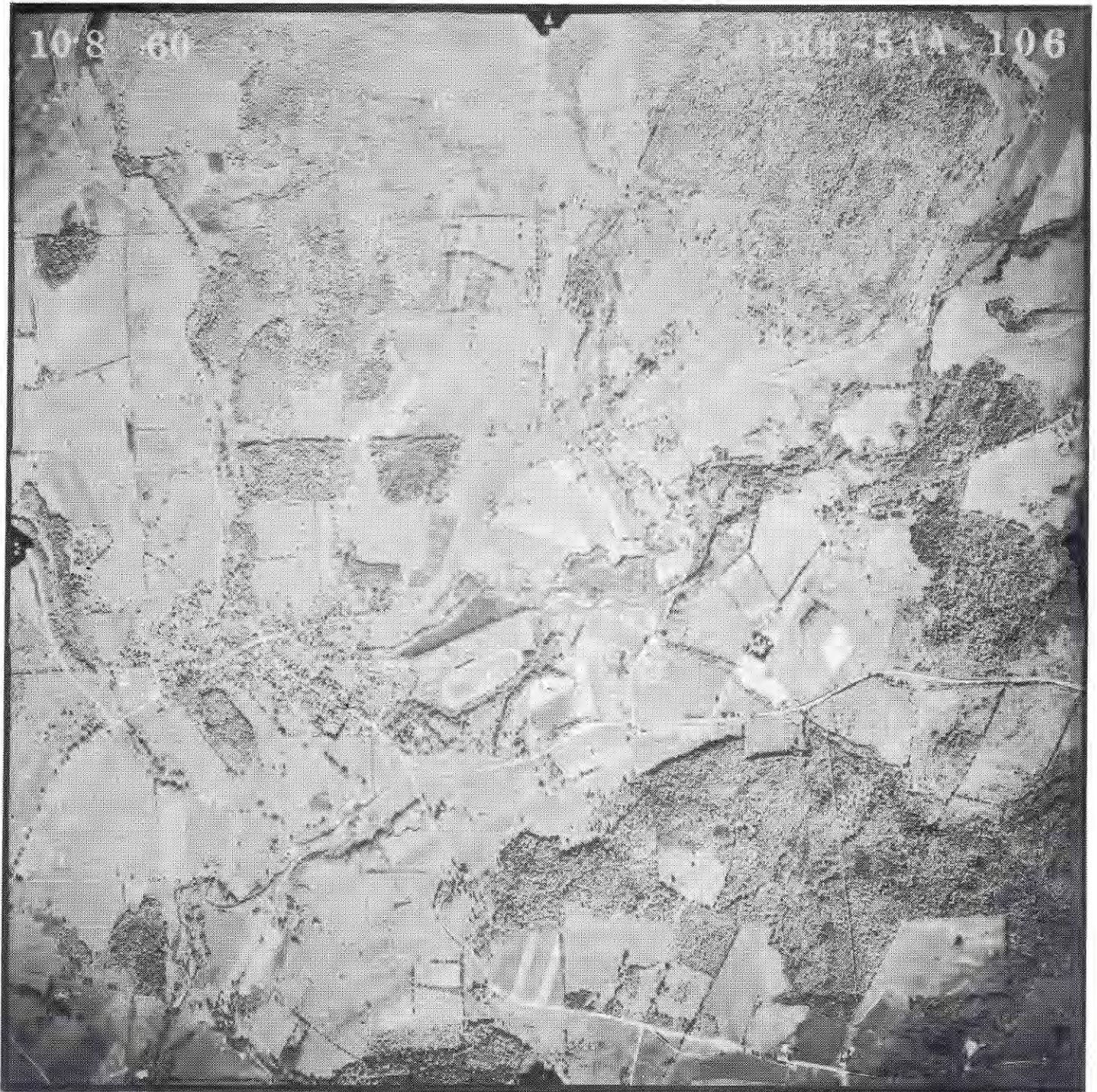
Example of an aerial photo from 1960 of an area including Morris, Otsego County. Much of the area that was cleared farm land in 1960 is today young forest land. Roads, edges of fields, mature forests, water bodies, hedgerows, and other key features, are easily identifiable from such photographs at low cost from the Farm Services Agency. Scale is 1"=1320.
