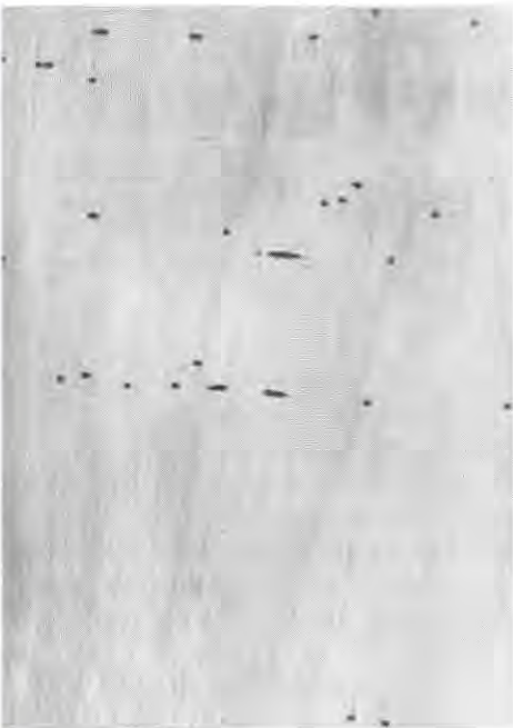
Fig. 3. Ambrosia beetle damage to yellow birch veneer. Actual dia. of each hole is 1 mm (.04 inches).
