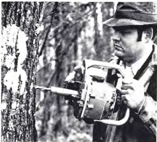
Drilling tap holes is made easier with drill modifications on chain saw power-plants.
