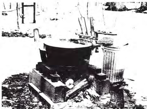
The backyard boiling setup with cinder block fireplace and washtub.
