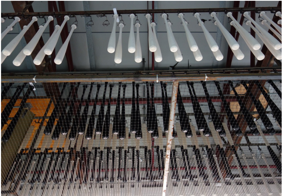
These bats have been dipped in paint or stain and then hung to dry
