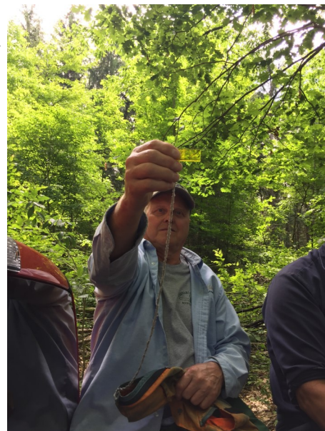
Chris Howard experimenting with Forester Bruce Robinson's Wedge Prism to determine basal area at the Burley woods walk.
