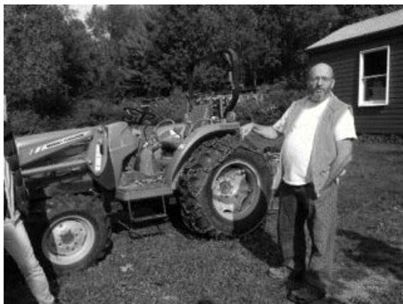
Charles cuts and moves firewood and sawlogs with the help of a Massey Ferguson model 1540, 40 hp, 4-wheel drive, and a 4 1/2 ton winch. The loader will
